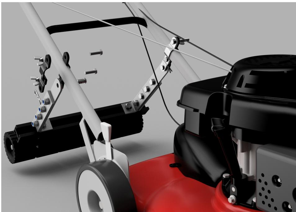
Once the Clamps are in place, begin tightening down. You want it to be snug and not able to pivot around the bar.
