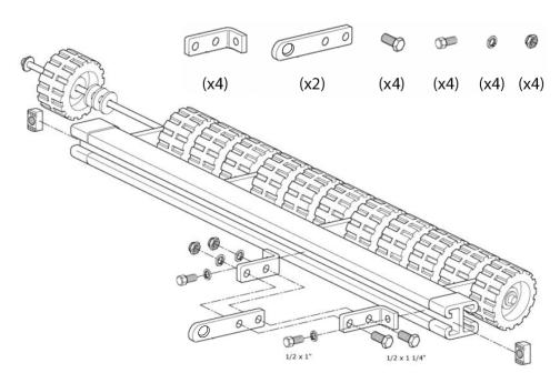
Step 4: Installing Striping Kit to Quick Release Brackets
