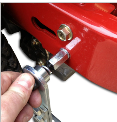
(5) Thread pivot bolt
