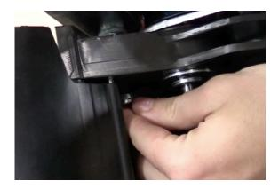
**Tighten**Using a 9/16" wrench and a 1/4" hex key, secure the mounting arm to the mower frame.
