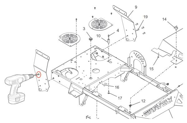
**Note:** Gravely Pro-Walk will require **two 3/8" Mounting Holes** (One on each side) to be drilled.
