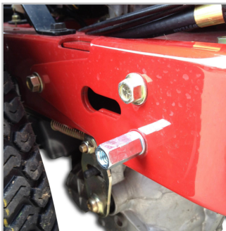
(4) Tighten coupler nut
