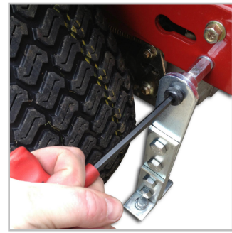
(6) Tighten pivot bolt
