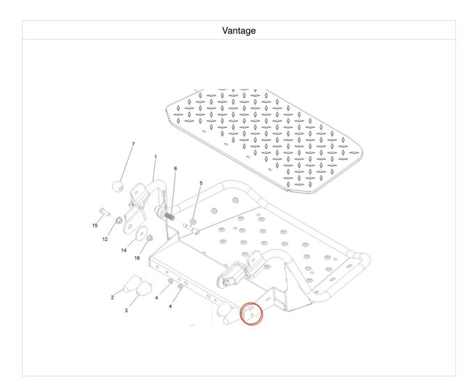
Pivot bolts mount directly into existing holes in the side of the operators platform.
