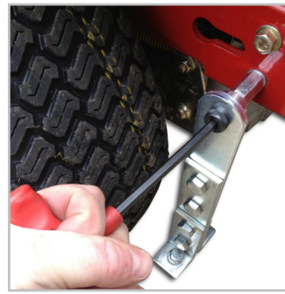
(6) Tighten pivot bolt
