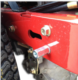
(4) Tighten coupler nut
