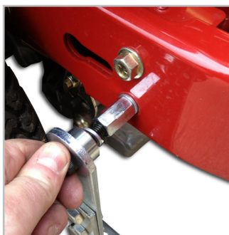
(5) Thread pivot bolt
