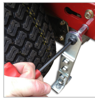
(6) Tighten pivot bolt
