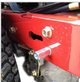
(4) Tighten coupler nut
