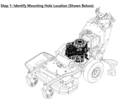
**Note:** Bad Boy Commercial Walk Behind will require **two 3/8" Mounting Holes** (One on each side) to be drilled.
