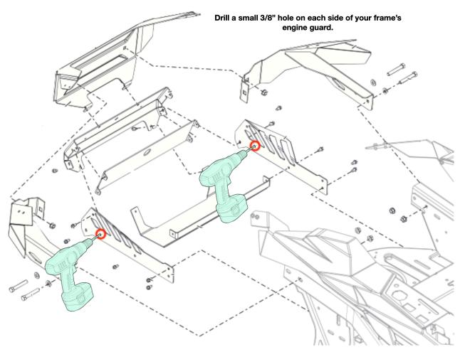
Each of these mowers require a single 3/8" hole to be drilled on each side at the rear of the frame. Reference the schematics for exact hole locations.
