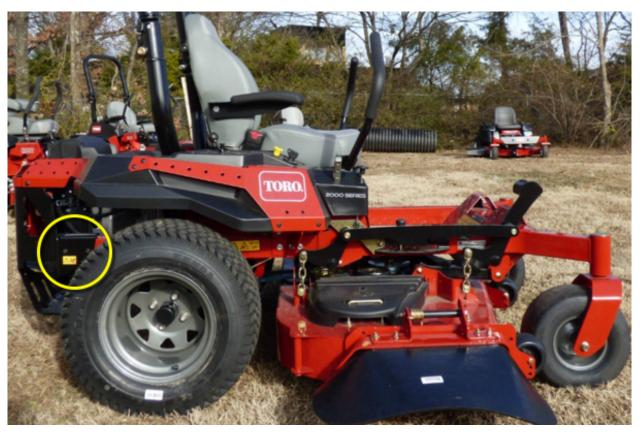
Note: Quick release pins MUST point in the same direction to allow the CheckMate™ Striping Kit to slide on and off from the pins. See example below:
