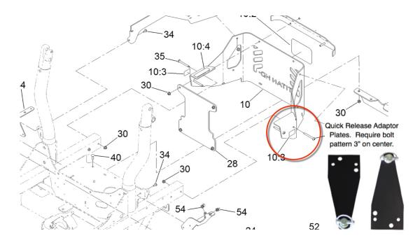
**Step 2:** Utilizing supplied  $3/8" \times 11/2"$  bolts, align quick release adaptor plate with existing holes/bolts in the side of the mower frame. Securely fasten adaptor plates to each side of the frame.
