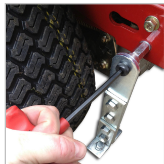
(6) Tighten pivot bolt
