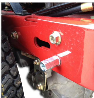
(4) Tighten coupler nut
