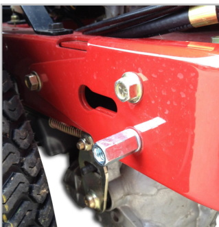
(4) Tighten coupler nut
