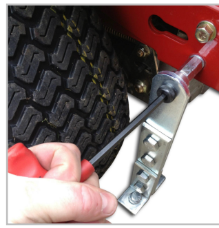
(6) Tighten pivot bolt
