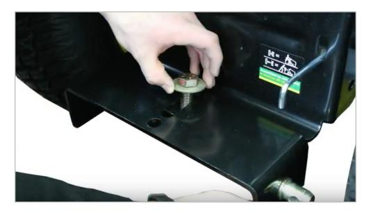
Step 3: Remove Quick Release Lynch Pins and Slide Mounting Arms onto Stabilizer Pins. Reinstall Lynch Pins.
