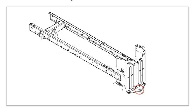
**Step 1:** Identify existing utility cart hole located at the rear of the tractor.
