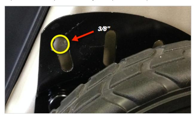
Step 3: Prepare to bolt Pivot Bolt to locking nut
