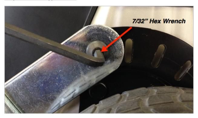
Step 5: Attach lower portion of mounting arm to roller
